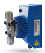
Kompact, even in its basic variant, uses premium materials in its manufacture. The **pump head** comes as standard in PVDF-T, but can be optionally specified in natural PVDF and comes with a ceramic ball valve as standard improving the reliability of the pump over time and offers chemical compatibility of the wetted parts. SEKO's diaphragms are made of pure solid PTFE offering a superior life expectancy guaranteed by SEKO for 5 years, making routine replacement no longer necessary.
