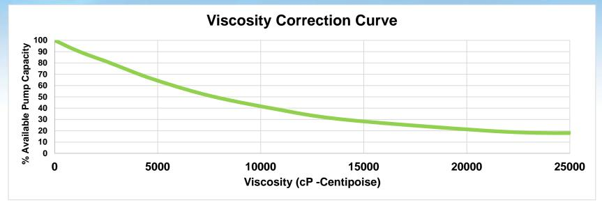
**Example:** 2" pump maximum flow on water = 156 gpm (590 lpm) Adjusted flow for 25,000 cP fluid = 156 gpm (590 lpm) X .2 = 31.2 gpm (118 lpm)
