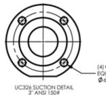
(4) Ø.63"(16.00mm) THRU EQUALLY SPACED ON A Ø3.88"(98.6mm) B.C.
