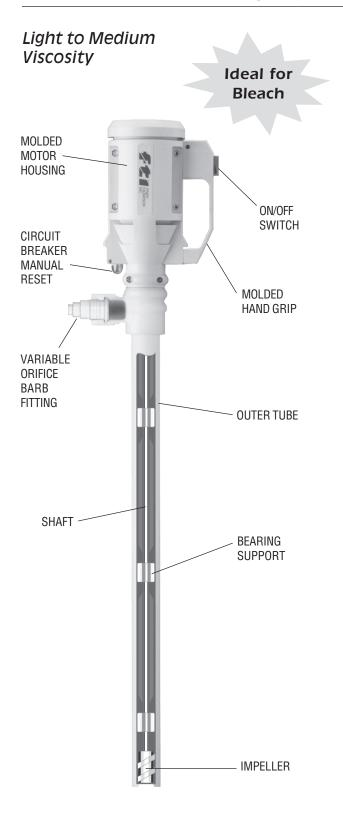
The TBP series is an economical, light to medium viscosity drum pump **constructed of pure materials** for use with bleach, nitric acids, hydrochloric acids, sulfuric acids, etc. The 1.66" (42mm) tube diameter is designed to accommodate drums with smaller bung openings. Typical applications include: Municipal water treatment facilities, swimming pool supply houses, water parks, anywhere that bleach is used in drums/barrels or containers.
